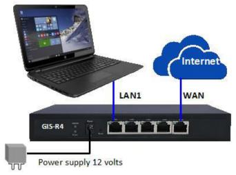
With your computer LAN port connected to the GIS-R4 LAN1 port open the computer browser, type 'aplogin.com'
