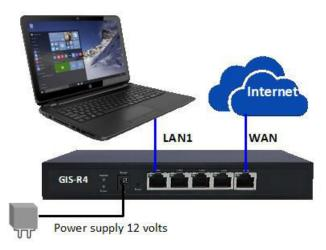
With your computer LAN port connected to the GIS-R4 LAN1 port open the computer browser, type 'aplogin.com'
