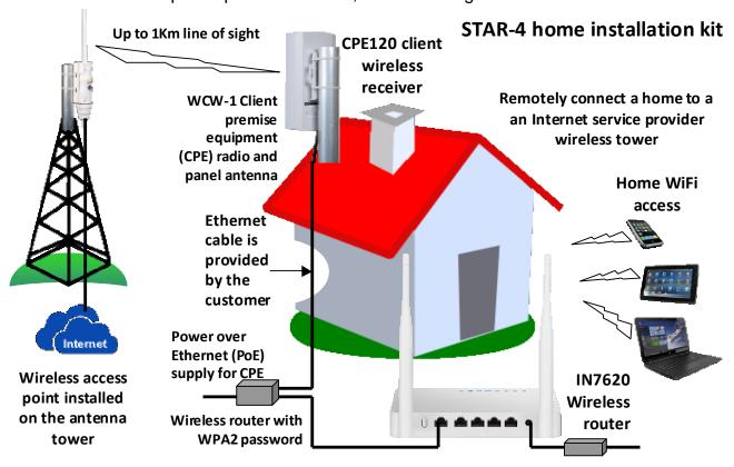
The pre-configured STAR-4 kit has two parts, the CPE120 wireless receiver that is installed on the home roof. This receiver must have a clear line of sight to the central wireless antenna. The CPE120 wireless receiver is connected to the IN7620 wireless router inside the home. The home residents connect WiFi devices to the IN7620 WiFi to get Internet access. The installer must provide the Ethernet cable that connects the CPE120 to the PoE power inside the home.
