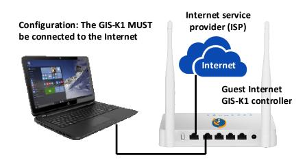
With your computer LAN port connected to the GIS-K1 LAN1 port open the computer browser, type 'aplogin.com'
