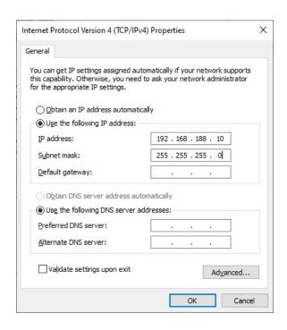
Finally click close. The LAN port can now be connected to the CPE120 products to configure them as a HOST or as a CLIENT.
