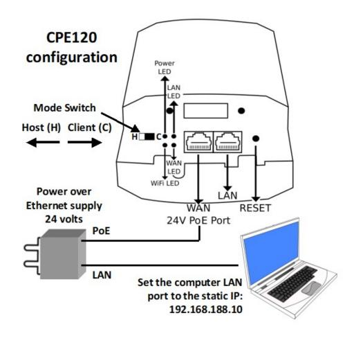
The Host or Client mode is selected using the switch shown in the diagram. When the mode has been selected then the configuration has to be made by selecting the parameters for that mode.
