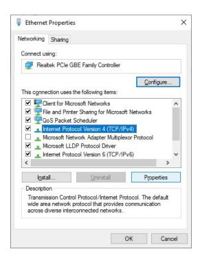
Select use the following IP address Enter the IP address: **192.168.188.10** Enter the subnet mask: 255.255.255.0 Click the OK button.
