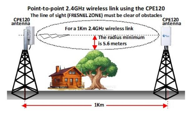
If the clearance is not provided the antennas will not communicate.
