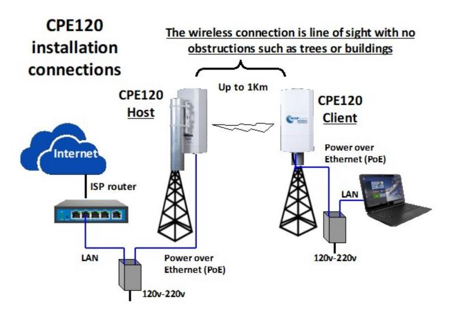
The CPE120 HOST connects to the Internet service using the Ethernet cable provided to connect the PoE supply to the ISP router.
