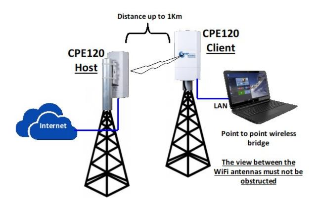
The CPE120 kit contains <u>two</u> wireless units, pre-configured as the HOST and CLIENT, see the diagram. A label on each product shows which is the HOST and which is the CLIENT. The products do not require configuration to install and operate them.
