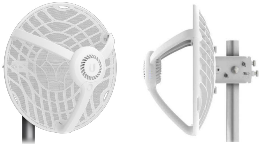
Figure 2.10.4. Wireless access point with antenna for the 61GHz unlicensed band. (Ubiquiti airFiber 60 LR. © Ubiquiti). The maximum transmission distance is 12Km.
