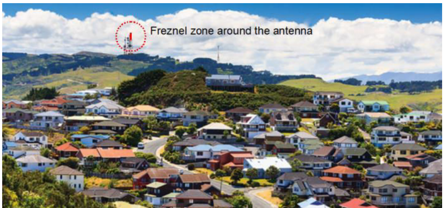
Figure 2.11.2. Clear space around the antenna for the Freznel Zone.
