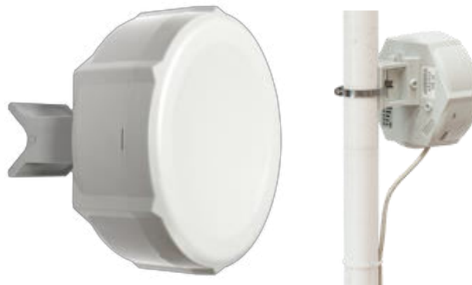
Figure 4.12.1. The Mikrotik SXT SA5 14dBi integrated Sector AP, 90 degrees beam-width, Gigabit Ethernet, with RouterOS that can have scripts added to function as an access controller when deployed together with a cloud-based WISP management system.
