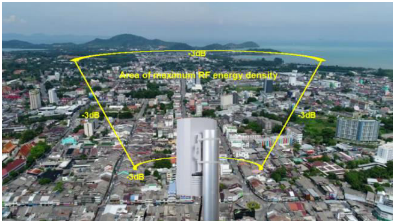
Figure 2.8.9. Panel directional antenna radiation field strength.
