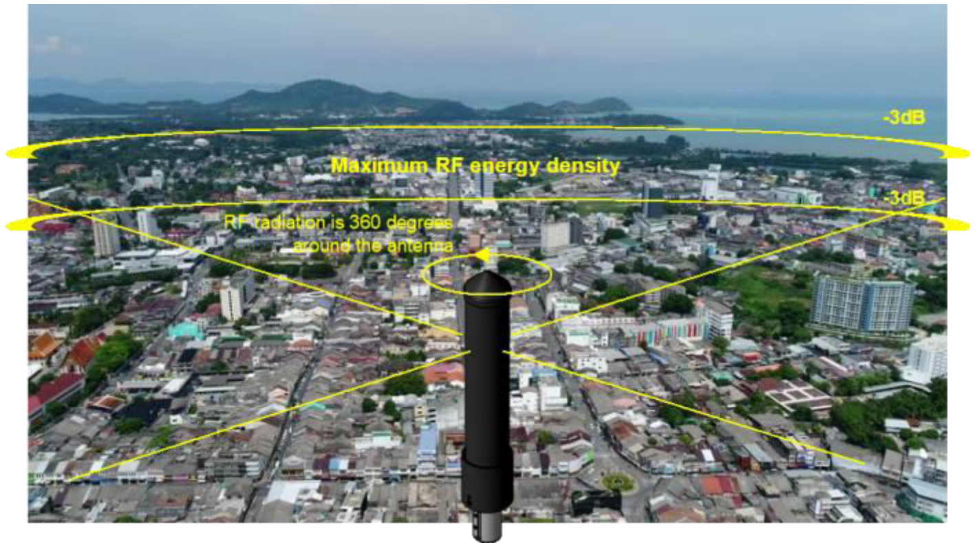
Figure 2.8.6. Down-tilt omni-directional antenna radiation field strength.
