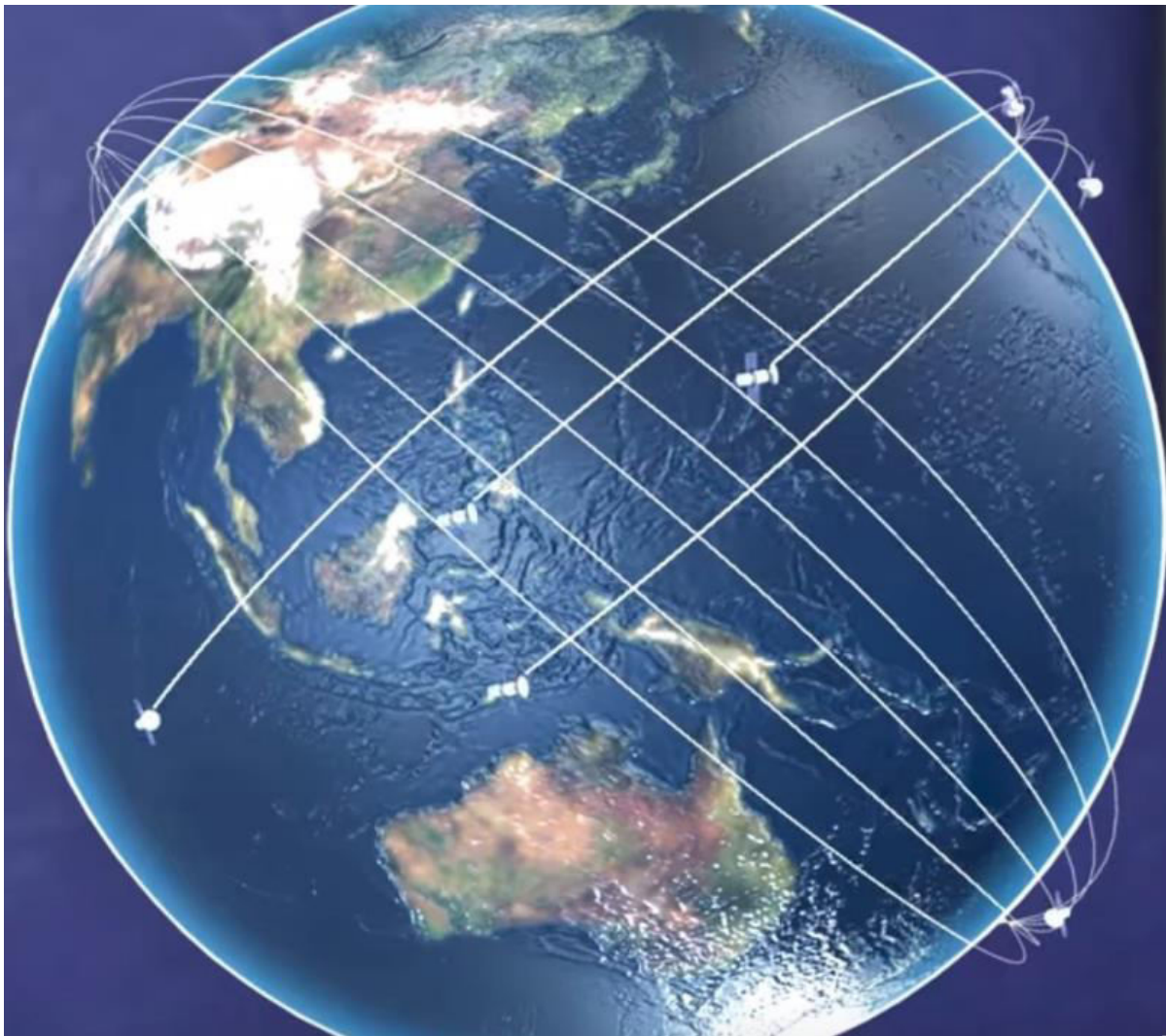
Figure 8.3.1. Starlink satellite orbital inclinations, within shells at different altitudes. (Image copyright © SpaceX 2021).
