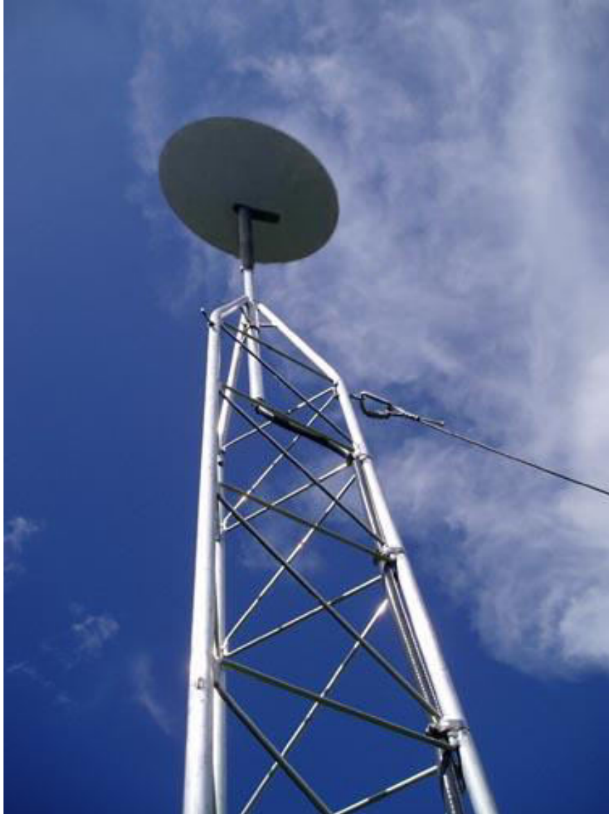
Figure 8.3.6. Starlink customer antenna mounted on a mast for a clear view of the sky (Image copyright © SpaceX 2021).
