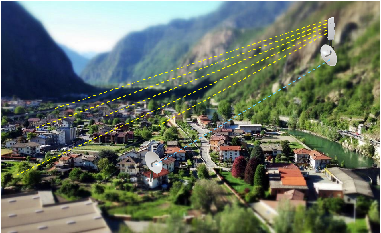
Figure 21: Wireless access point installed on a hillside and connected to an Internet service provider over a point-to-point wireless link.
