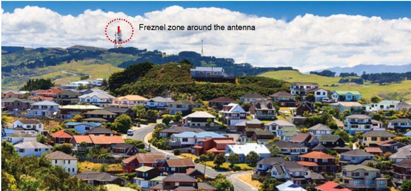
Figure 18: Clear space around the antenna for the Freznel Zone.
