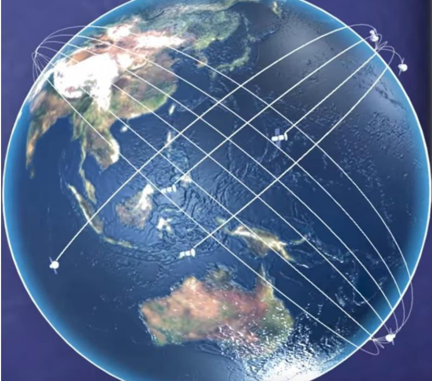
Starlink satellite orbital inclinations; within shells at different altitudes. (Image copyright © SpaceX 2021).
