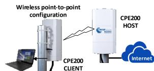
Point-to-point 5.8GHz wireless link using the CPE200 The line of sight (FRESNEL ZONE) must be clear of obstacles
