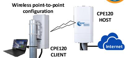
Point-to-point 2.4GHz wireless link using the CPE120
