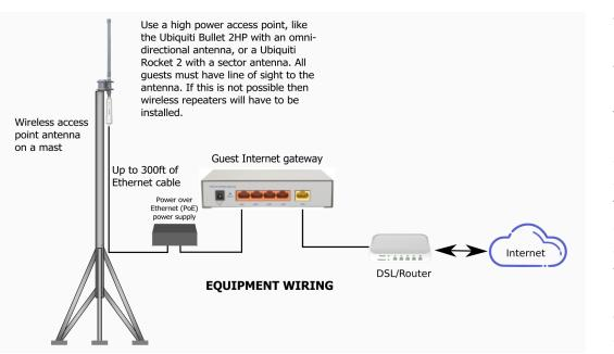
The Guest Internet gateway is installed in the main office together with the DSL or Cable router. An Ethernet cable runs from the gateway LAN port to the power injector for the wireless access point, and then along another Ethernet cable up to 300 feet in length. This cable runs up a tall mast with the wireless access point installed at the top of the mast. The wireless access point should be above the height of adjacent trees to ensure good signal transmission.
